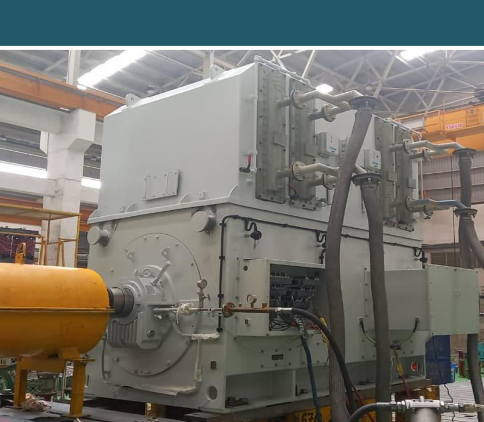
MOTOR COOLER 150 KW X 4 sections
